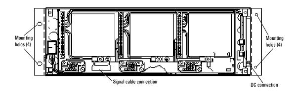
Figure 2 · MPS75 Modular Power shelf · NT5C10C with 26-pin signal connectors
